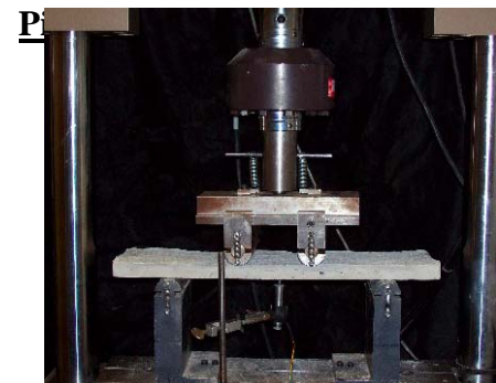
Figure 2 and 3: Third-point Load-Deflection Results and Setup for Plate with Fiberglass mesh
