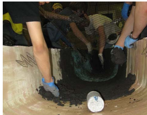
Figure 6: Canoe Placement, Note Placement of Mesh between Layers
