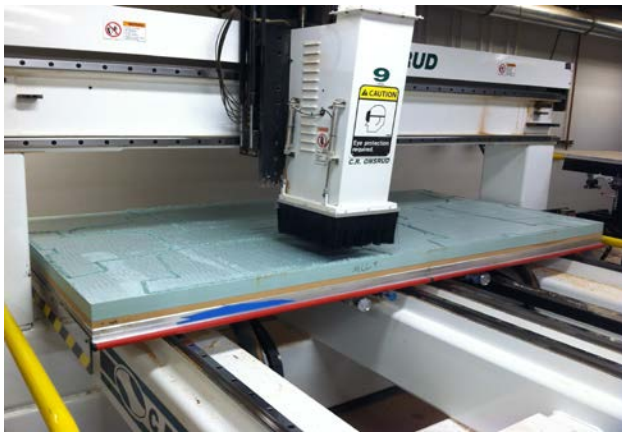
Figure 9: Cutting the foam mold using a 3-axis CNC router.
