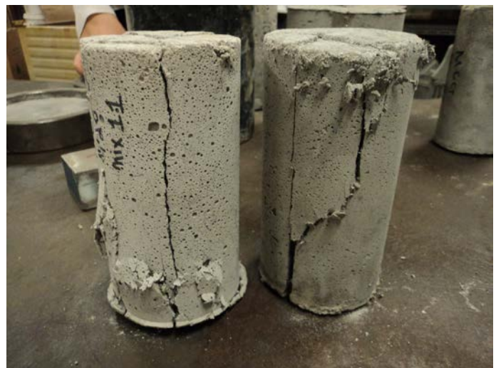
Figure 8: Cylinders of test mixes after compression testing.
