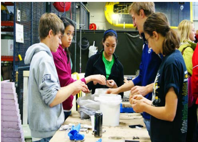
Figure 7: Separating fibers to use in varying proportions in test mixes.
