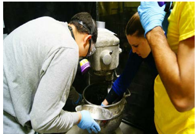
Figure 6: Mixing aggregate and cementitious material with admixtures.
