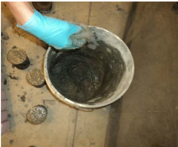
Figure 5: Concrete cylinders being formed for testing.
