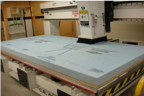
Figure 9: Cutting out male mold using CNC router.
