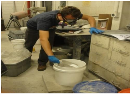
Figure 5: Measuring aggregates and cementitious materials.
