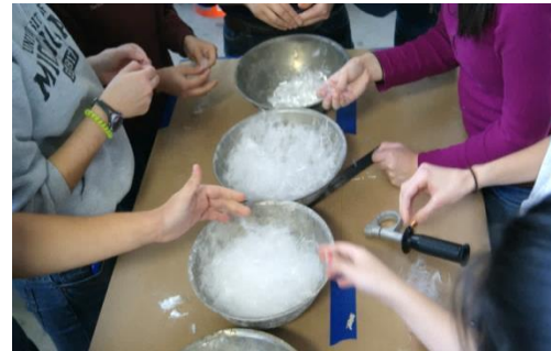
Figure 8: Separating fibers for varying proportions in each test mix.
