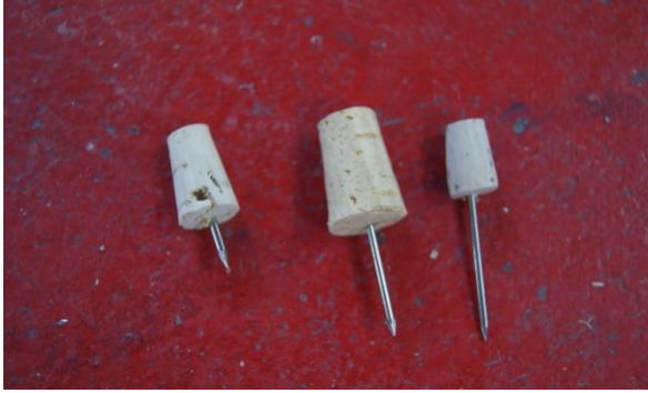
Figure 11: Three sizes of quality control devices for hull thickness measurement.
