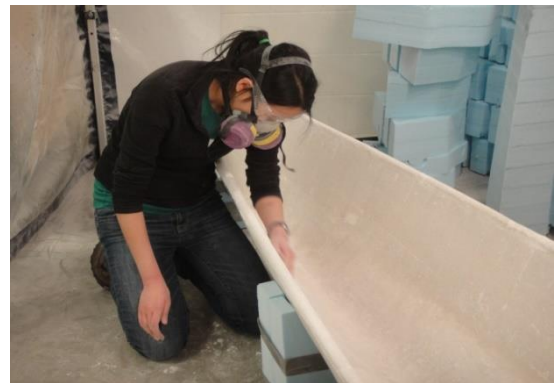
Figure 13: Hand sanding the interior of LEGACY after demolding.
