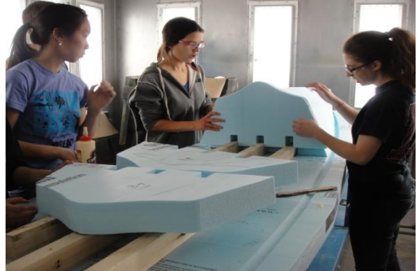
Figure 10: Aligning mold pieces on 2" x 4" beams.
